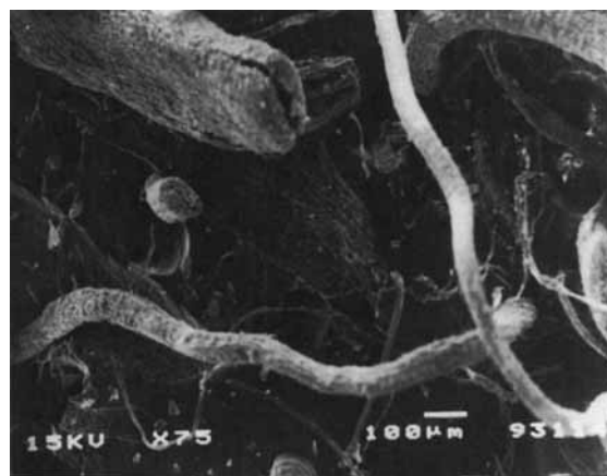
Figure 9 SEM of fractured end of tear specimen of mix G: shows no fiber pullout, which indicates better fiber-rubber adhesion.
